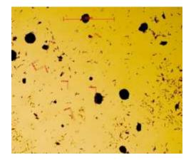
Poor filtration batch: Fines resulted in agglomeration
