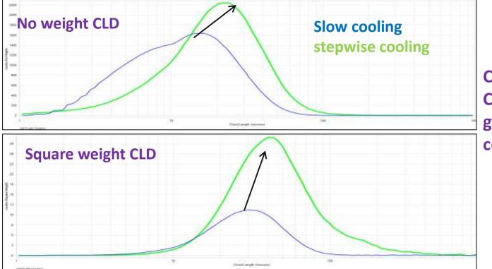
Comparing both the CLDs indicate particle growth during the cooling crystallization
